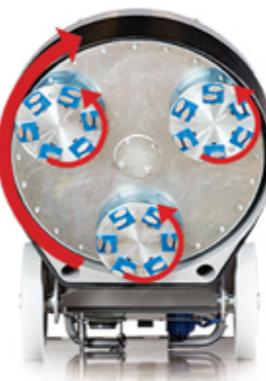
Figure 4-1 Illustrates the rotation of the grinding heads versus the gear barrel.
