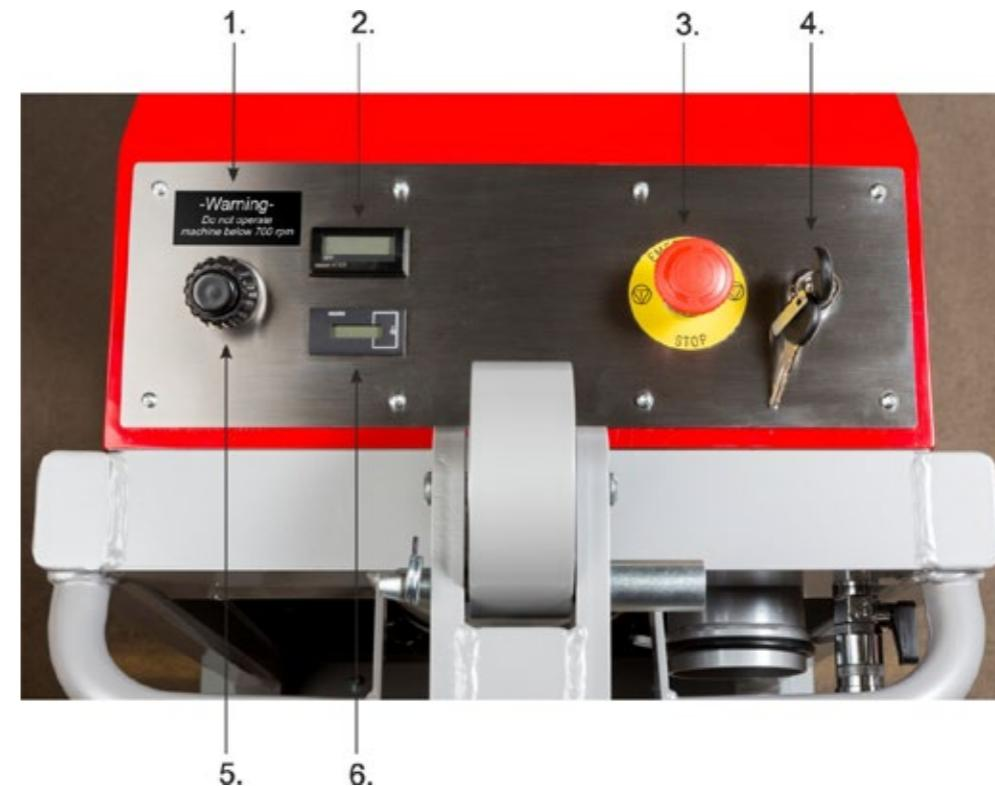
Figur 4-5 Kontrollpanel SC-800 Propane
